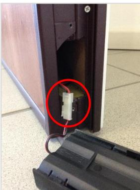
3. Remove the battery pack disconnecting the 2 poles connector.
