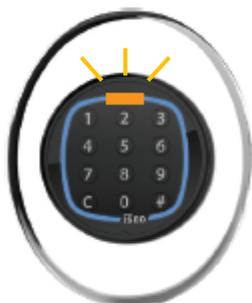
This operation, that **keeps about 20 seconds**, is indicated to the user by the orange led, in the external module, continuously flashing.
