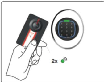
1. Present the *Master Card* 1 to the device to enter in *Programming Mode*.
