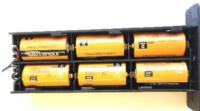
5. Replace all batteries with the right model: 6x1,5V alkaline batteries "D" type.
